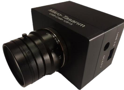
Figure 7. Modular USB camera called USB-CAM-12815 built to demonstrate the imaging performance of MT12815CA-3G ROIC with SWIR detector arrays. The camera has a 50 mm f/1.4 C-mount SWIR lens with manual aperture and focus control. The camera has a USB 3.0 interface, measures 90 mm  $\times$  65 mm  $\times$  55 mm, and weighs 275 gr without the lens.
