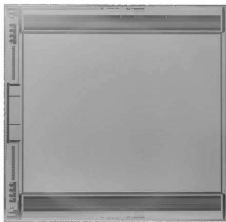
Figure 3. Die photograph of MT12815CA-3G ROIC. It measures 21.8 mm × 21.1 mm in a 180 nm mixed-signal CMOS process.
